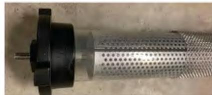
Figure 1. Corona discharge tube.
